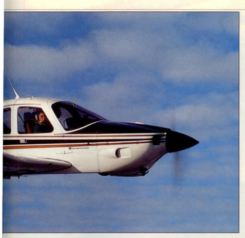
never could get the doors to seal properly, and finally in 1974, two years after the 112 debuted, the company announced the 112A. The most pronounced differences between the two were in the doors. The 112A used metal doors that solved the air leak and resulting noise problem caused by the fiberglass ones. The new designation also carried a 100-pound gross weight increase to 2,650 pounds and an improved ventilation system.
